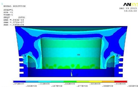
Figure 5: Thermal stress on the piston
