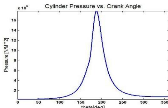
Figure 2: Pressure variation with crank angle
