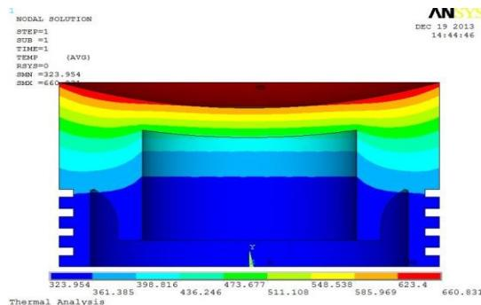
Figure 3: Temperature distribution over the piston.
