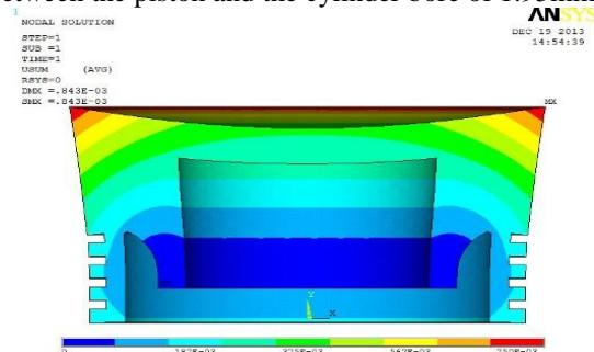
Figure 4: Piston deformation under thermal load
