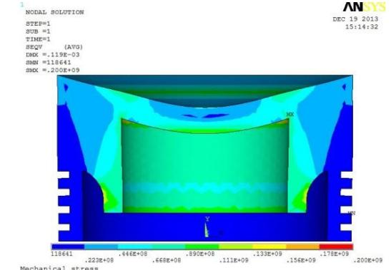
Figure 7: Mechanical stress on the piston
