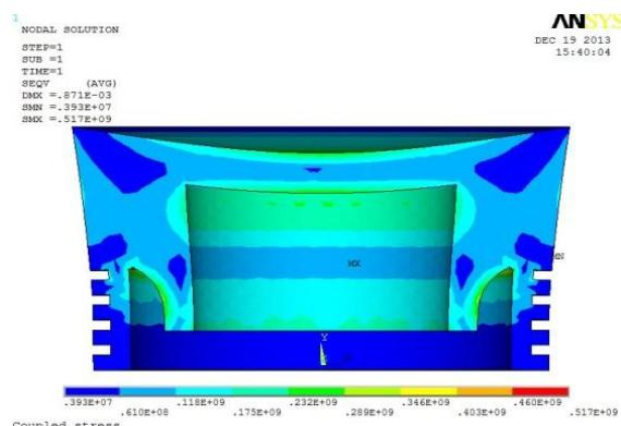
Figure 9: Coupled Thermal-Mechanical stress on the piston
