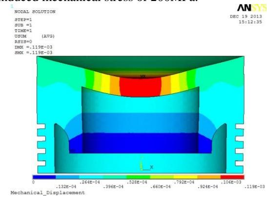
Figure 6: Piston deformation under mechanical load
